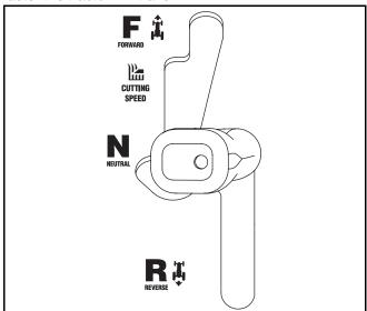
Place the speed control lever in the Cutting Speed, or slower, position when mowing.
